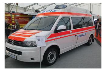
Basic colour is white and paintable also in different colours. Spoiler is made of GRB (glass-reinforced plastic). Lenses are made of polycarbonate This solution fits into the Volkswagen T5 factory high roof. Product is Surface mount-ing version and easy and fast to install.
